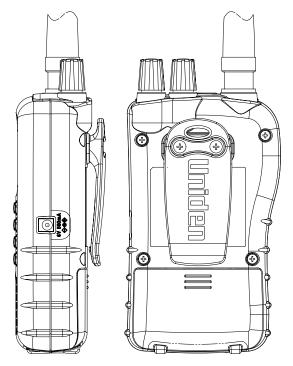
To make your scanner easier to carry when you are on the go, use the supplied belt clip. Use a Phillips screwdriver and the supplied screws to attach the clip to the scanner.
